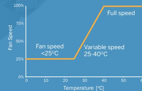
EcoPower will analyse the temperature and humidity conditions and automatically select the profile with the highest fan speed
